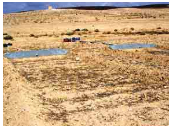
Photo 2.2. A pair of constructed runoff plots with collection tanks.
