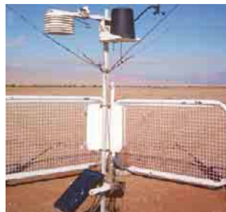
Photo 2.1. Hobo automatic weather station at Mharib site.
