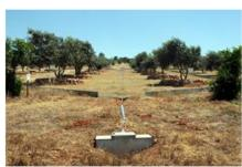
Measuring water runoff from experimental plots.
