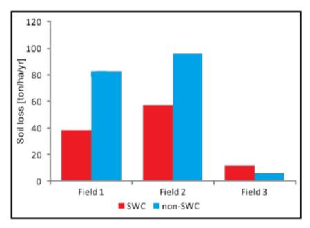
Figure 12: Soil loss for fields with and without SWC interventions
