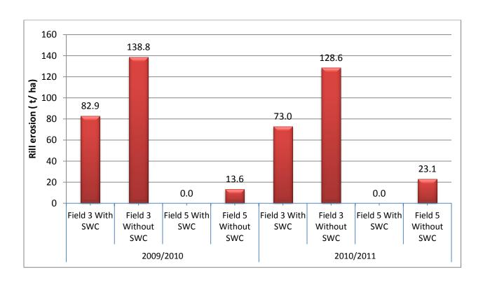
Figure 10: Comparison of rill erosion for fields with and without SWC interventions during two rainy seasons
