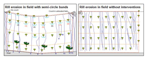
Figure 9: A sketch showing the distribution of rills in a field with semi-circular bunds and a field without any interventions
