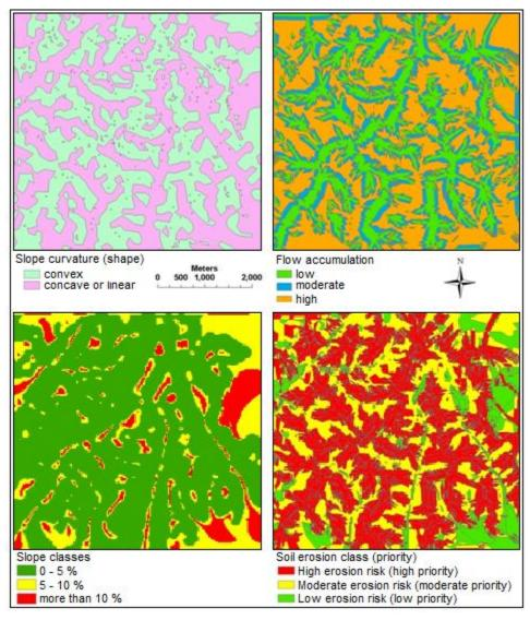
Figure 4: Overlays of flow accumulation, slope, and curvature maps used to produce the land degradation priority map
